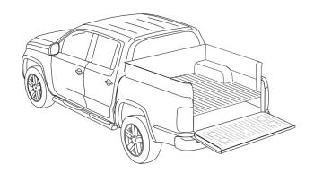
4. Locate and align the pre-drilled holes in the truck cargo bed and the bedliner, then insert the scrivets.
